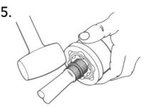
Most other outboard C.V. Joints are held on to the axle shaft with an internal snap ring. These C.V. Joints can be removed by striking the joint face with a mallet.
